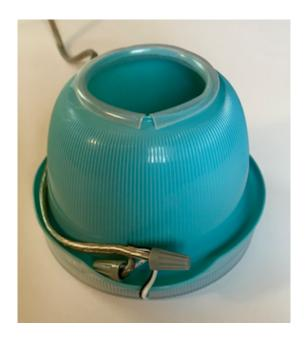
Tuck the two wire nuts into the bottom of the cup handle and secure them with a hot glue gun. You can also secure part of the speaker wire under the cup lip using the hot glue.
