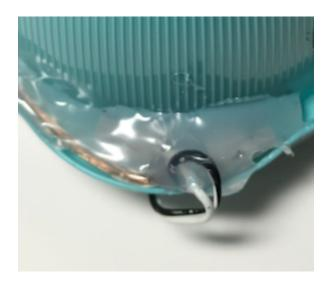
Apply velcro strips with the sticky backing to two sides of the cup. Use the non-fuzzy type of velcro for the cup sides. Cut two lengths of hook loop strap type of velcro and attach them to either side of the cup to form an adjustable hand strap with the fuzzy side against the top of the hand used to hold the Pulsar.
