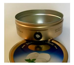
Cut an extra long length of speaker wire. Pull the conductors apart at one end, strip off 1/4 inch of insulation on both ends, and attach them to the transducer. The transducer uses the same type of clamp connectors as the audio amp. Thread the cable through the grommet in the tin.
