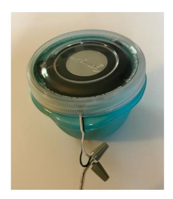
Using a hobby knife blade, cut out the bottom of the Rubbermaid cup up to but not including the bottom ridge. Cut a length of 1/4" tubing and, using the hobby knife blade, cut a slit along its entire length. Install the tubing over the cup's bottom ridge and edge.
