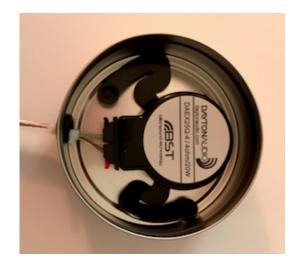
To cut down on handling vibrations cut out a pad of foam and attach it with glue or tape to the top of the tin.
