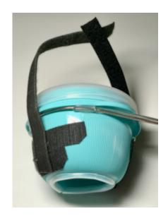
To cut down on handling vibrations cut out a pad of foam and attach it with glue or tape to the top of the cup.
