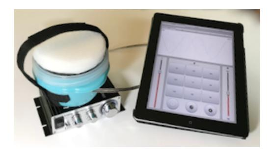
This enclosure is designed to transmit less of the mechanical vibration of the transducer and more of the acoustic air waves. It is thought that mechanical waves stay at the surface of the body while the acoustic waves are better able to penetrate into the body.
