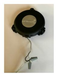
Use a file to cut a slot through both the tray insert and the lid edge of the cup. Position the slot over the cup handle. Feed the transducer wires through the slot before screwing on the lid. The transducer is now completely enclosed in the top of the cup.
