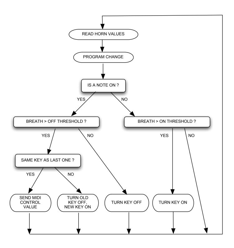
FIGURE 4 - Program Flow Diagram
