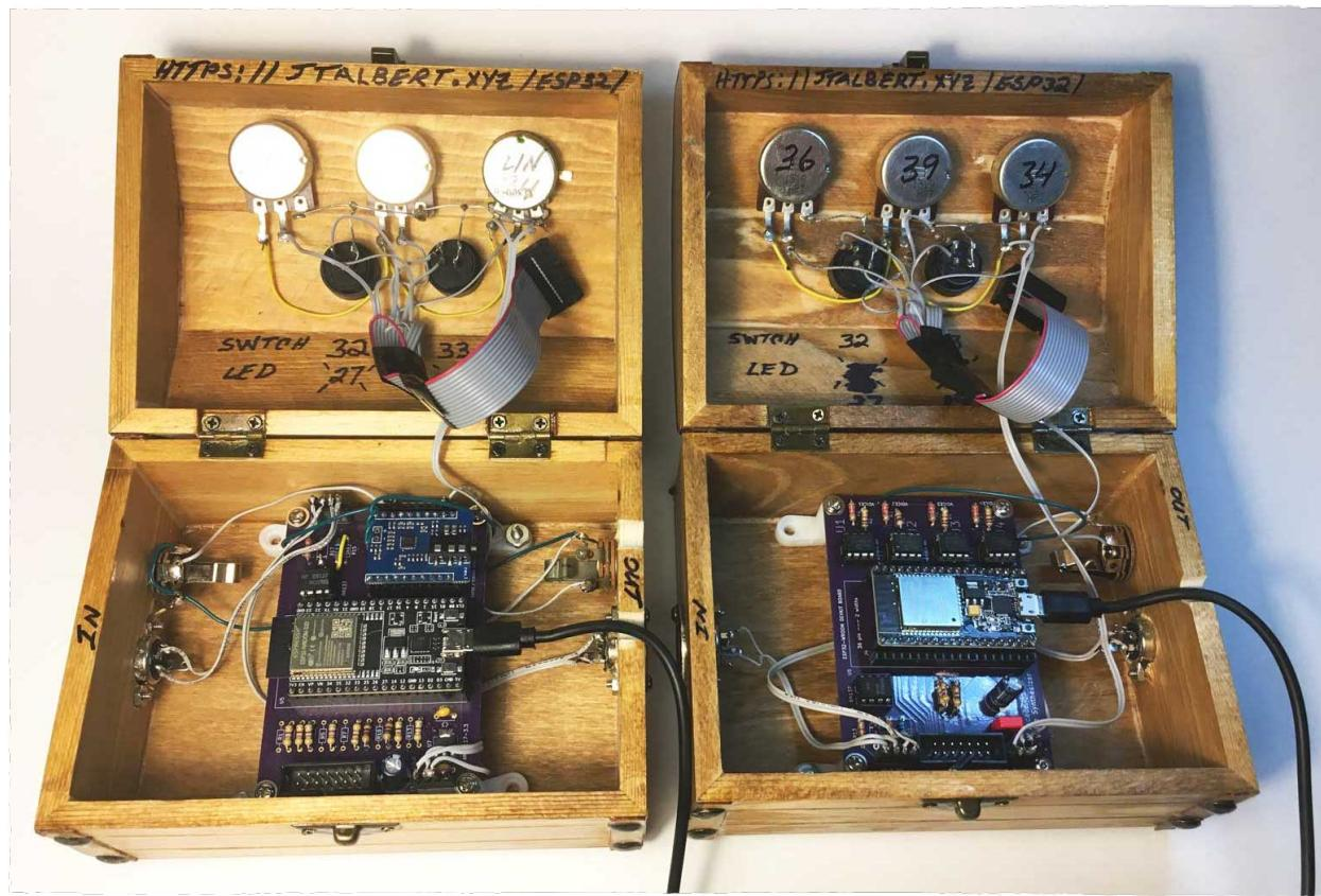
The circuits are shown here. Note the 470 Ohm resistor used in the Switch and Potentiometer circuits. This small resistor protects the micro pin from short circuiting to Ground in the event the pin is mistakenly programmed as an output instead of an input.
