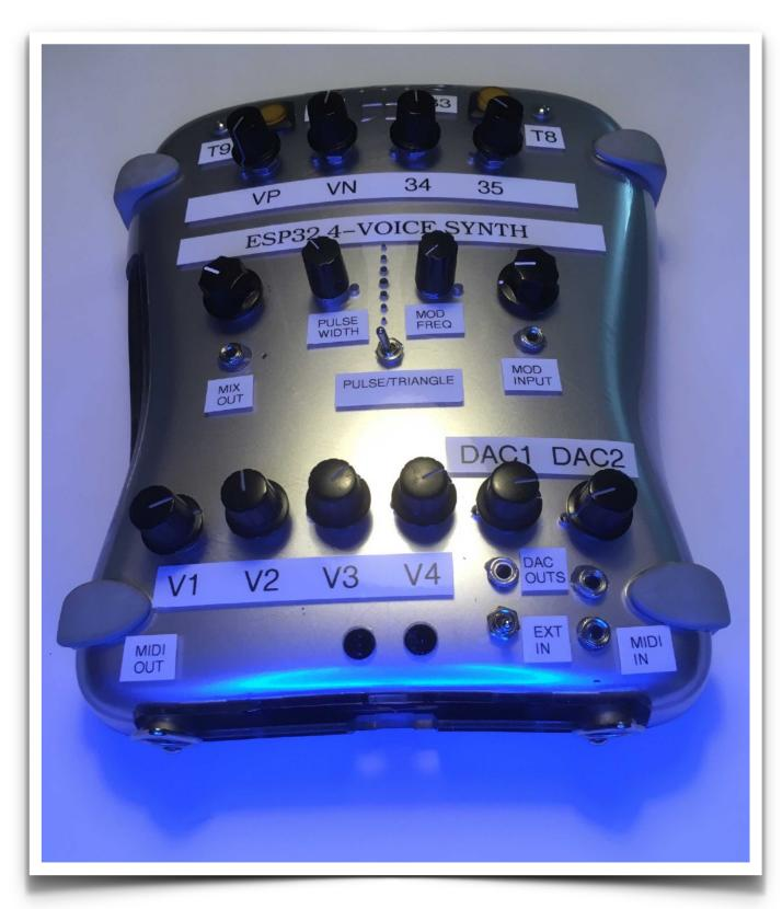
Here is the AY ESP32 Synthesizer built into a chassis. All 4 voices from the PCB are used along with the two extra X1 and X2 pins for a total of six. Volume controls are provided for all six voices at the bottom of the box. A switch is put on one of the ESP32 DAC voices to allow a choice between the DAC and any external signal to be added to the mix. Output jacks are provided for each of the ESP32 DAC signal pins (before volume control).
