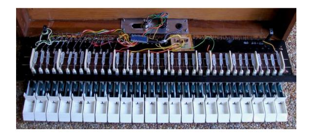
Each key is connected to a flexible spring that is pulled and slightly stretched across a metal bar when the key is depressed. The metal bar covers the entire length of the keyboard but is electrically segmented into 4 separate "busses" each of which covers one octave or 12 keys. One
